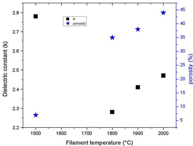
Fig. 5. Effect of filament temperature on dielectric constant (k) and porosity (%).
