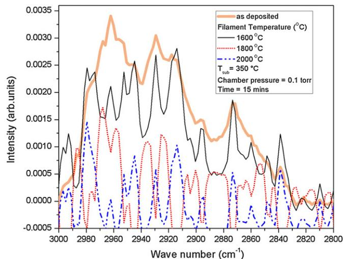
Fig. 1. FTIR spectra (for 1600, 1800 and 2000 °C) in the region  $2800$ – $3000\text{ cm}^{-1}$  showing the influence of the filament temperature on the concentration of remaining  $\text{C}-\text{CH}_x$  groups after a 15 minute atomic H treatment of the SiOC:H film.
