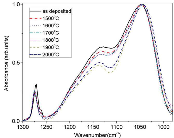
Fig. 2. FTIR spectra of the Si–O, and Si– $\text{CH}_3$  bonds in the region  $1000$ – $1300\text{ cm}^{-1}$  showing the influence of the filament temperature of a 15 minute atomic H treatment of the SiOC:H film.
