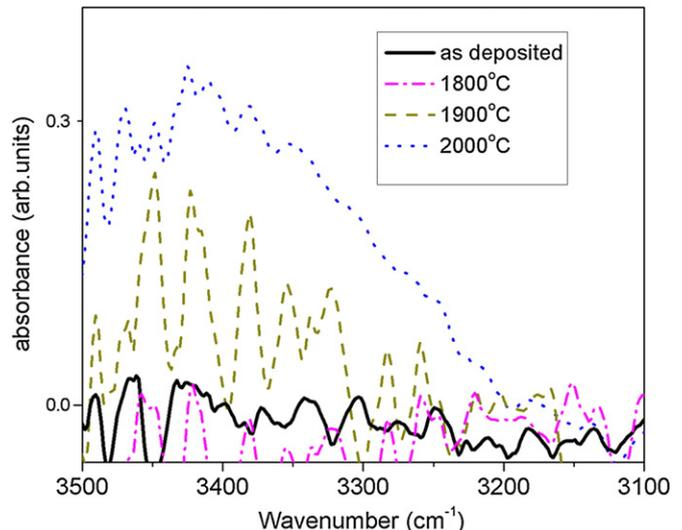
Fig. 3. FTIR spectra of  $-\text{OH}$  bonds in the region  $3100$ – $3500\text{ cm}^{-1}$  for samples treated at filament temperature of 1800, 1900 and 2000 °C.
