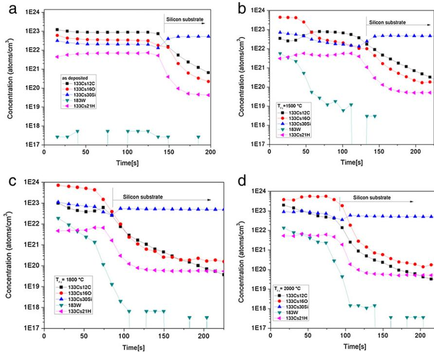
**Fig. 4.** SIMS profile of the elements Si, O, C that compose the SiOC:H film, also W (coming from the W wires) profile for 4 conditions : (a) as deposited films, (b) after atomic H treatment at filament temperature 1500 °C, (c) after atomic H treatment at filament temperature 1800 °C, (d) after atomic H treatment at filament temperature 2000 °C.
