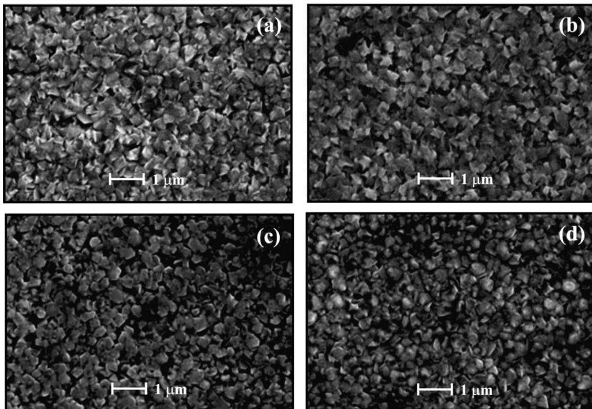
**Fig. 2.** SEM images of ultrasonically sprayed ZnO thin films with different water contents (a) 0 ml, (b) 2 ml, (c) 5 ml, and (d) 10 ml.
