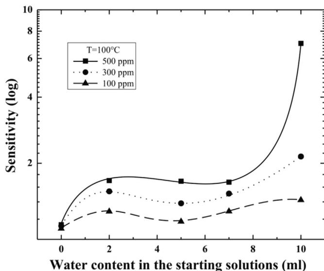
Fig. 3. Sensitivity of propane gas with respect to water content in the spraying solution measured at 100 °C for 100, 300 and 500 ppm.
