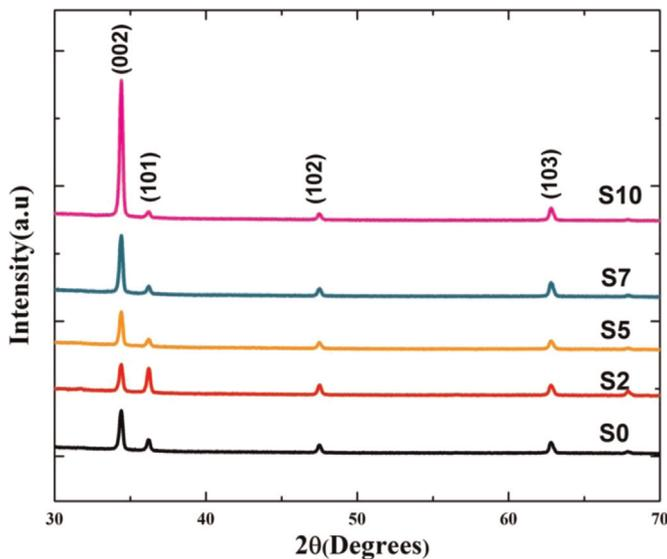
**Fig. 1.** XRD of ultrasonically sprayed ZnO thin films.
