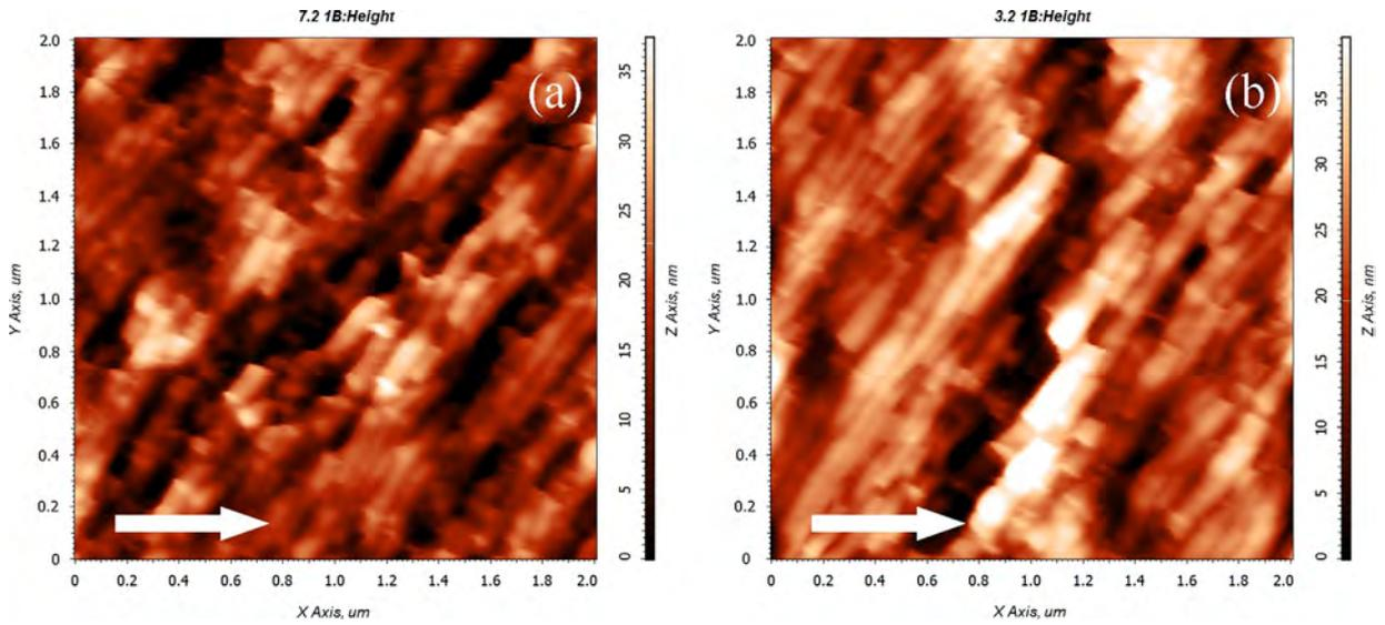
**Fig. 4.** 3D surface of GaSb after bombardment with 500-eV oxygen ions using different ion fluences: (a)  $2.5 \times 10^{18}$  ions/cm<sup>2</sup>; the maximum height is 45 nm and (b)  $5 \times 10^{18}$  ions/cm<sup>2</sup>, the maximum height is 70 nm. The angle of the incident ion beam is 45°. Image size is  $5 \times 5 \mu\text{m}^2$ .
