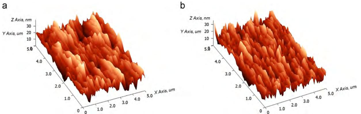
**Fig. 3.** 3D surfaces of GaAs after ion bombardment with oxygen ion beam at 45° incidence. The ion beam energy is 2 keV, ion fluences are  $3.125 \times 10^{18}$  ions/cm<sup>2</sup> (a) and  $5.4 \times 10^{18}$  ions/cm<sup>2</sup> (b). The images size is  $5 \times 5 \mu\text{m}^2$ .
