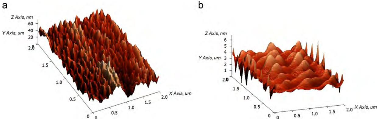
**Fig. 8.**  $2 \times 2 \mu\text{m}^2$  micrographics in 3D of InSb surface after ion bombardment at a  $45^\circ$  incidence angle using a 2 keV oxygen ion beam at ion fluences  $2.5 \times 10^{18}$  ions/cm<sup>2</sup> (a) and  $1.5 \times 10^{19}$  ions/cm<sup>2</sup> (b).
