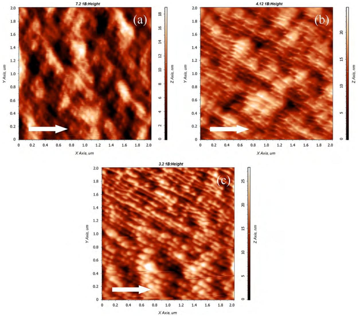
**Fig. 2.**  $2 \times 2 \mu\text{m}^2$  images of GaAs surfaces bombarded with  $\text{O}_2^+$  ion beam, the ion energy remains constant at 1 keV and the ion fluence is different for each case: (a)  $1.5 \times 10^{18}$  ions/cm<sup>2</sup>, (b)  $1.8 \times 10^{18}$  ions/cm<sup>2</sup>, and (c)  $6.2 \times 10^{18}$  ions/cm<sup>2</sup>. The white arrow indicates the direction of the ion beam at a 45° incidence angle.
