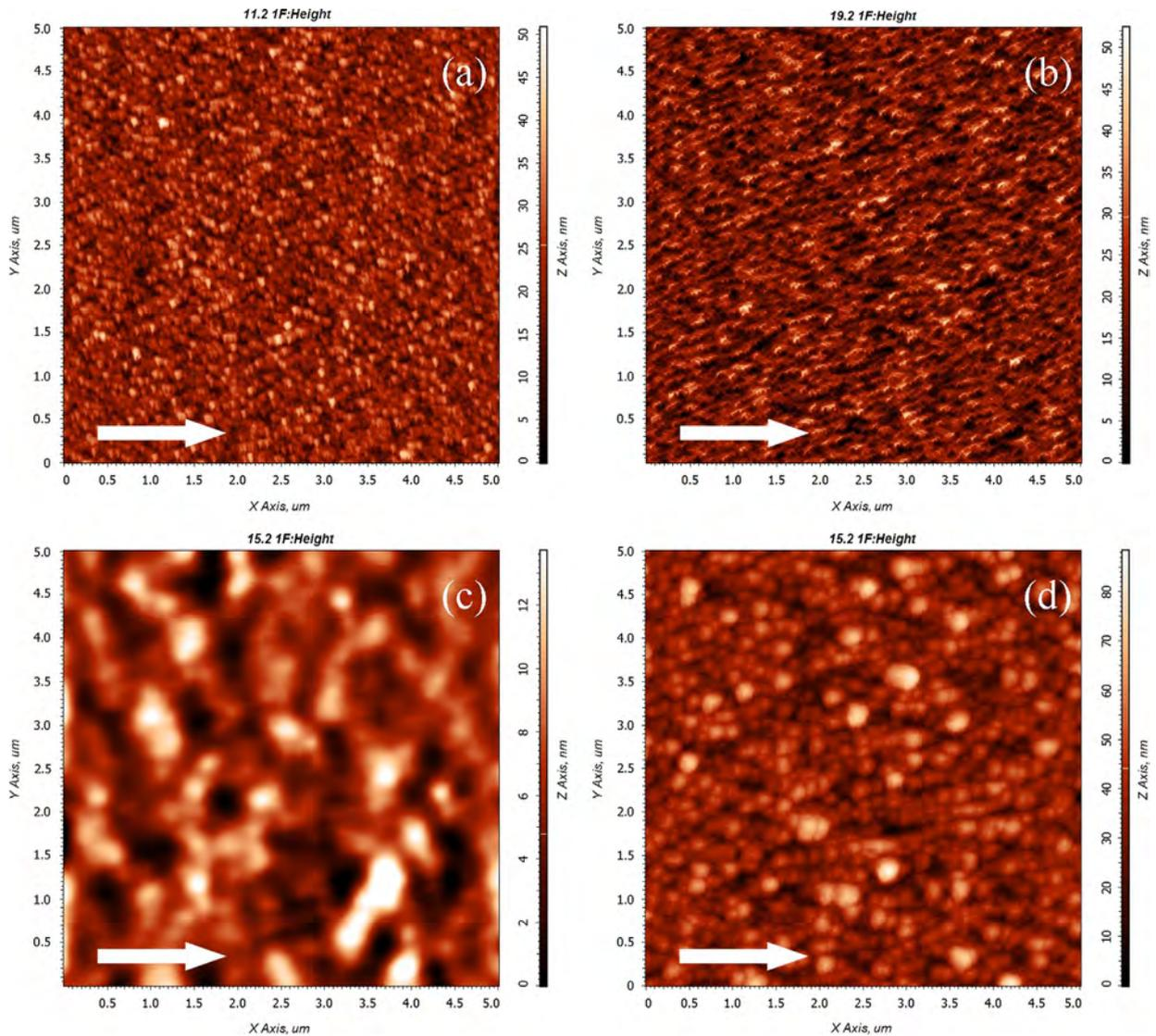
**Fig. 10.** AFM images, showing a sequence of the evolution of InSb surface topography with increasing the ion fluence: (a)  $4.2 \times 10^{17}$  ions/cm<sup>2</sup> (b)  $6.2 \times 10^{17}$  ions/cm<sup>2</sup> (c)  $1.2 \times 10^{18}$  ions/cm<sup>2</sup> (d)  $2.5 \times 10^{18}$  ions/cm<sup>2</sup>. The ion energy is 500 eV and the angle of incidence is 45°. The images size is  $5 \times 5 \mu\text{m}^2$ .
