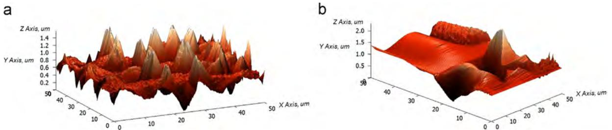
**Fig. 7.** 3D surface of InSb after ion irradiation with  $O_2^+$  ions. The angle of incidence is  $45^\circ$  and the ion energy is 2 keV. Sputtering fluence is:  $3.7 \times 10^{18}$  ions/cm<sup>2</sup> (a) and  $1.5 \times 10^{19}$  ions/cm<sup>2</sup> (b). Image size is  $50 \times 50 \times 5 \mu\text{m}^3$ .
