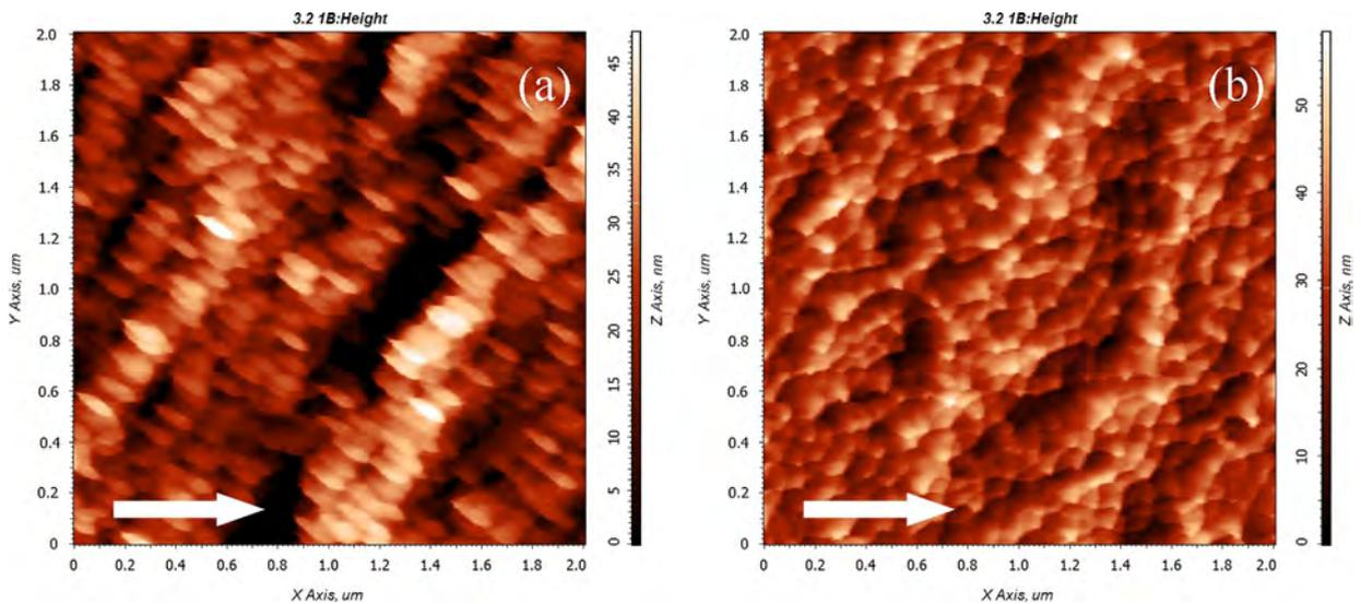
**Fig. 5.**  $2 \times 2 \mu\text{m}^2$  AFM image of a GaSb surface after ion bombardment by  $\text{O}_2^+$  ions at 45° incidence angle using different ion energies and ion fluences: (a) 1 keV, the ion fluence is  $6.2 \times 10^{18}$  and (b) 2 keV, the ion fluence is  $5.4 \times 10^{18}$ .
