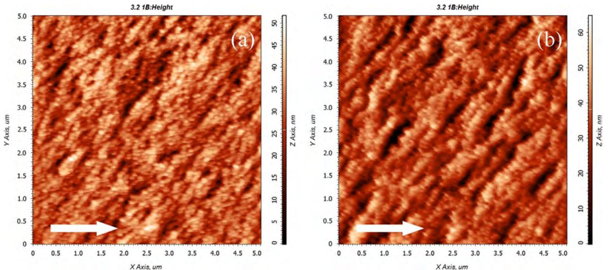
Fig. 6.  $5 \times 5 \mu\text{m}^2$  AFM images of eroded GaSb by 1-keV oxygen ions for different ion fluences:  $3.1 \times 10^{18}$  ions/cm<sup>2</sup> (a) and  $6.2 \times 10^{18}$  ions/cm<sup>2</sup> (b). The angle of incidence is 45°. The white arrow shows the ion beam direction.
