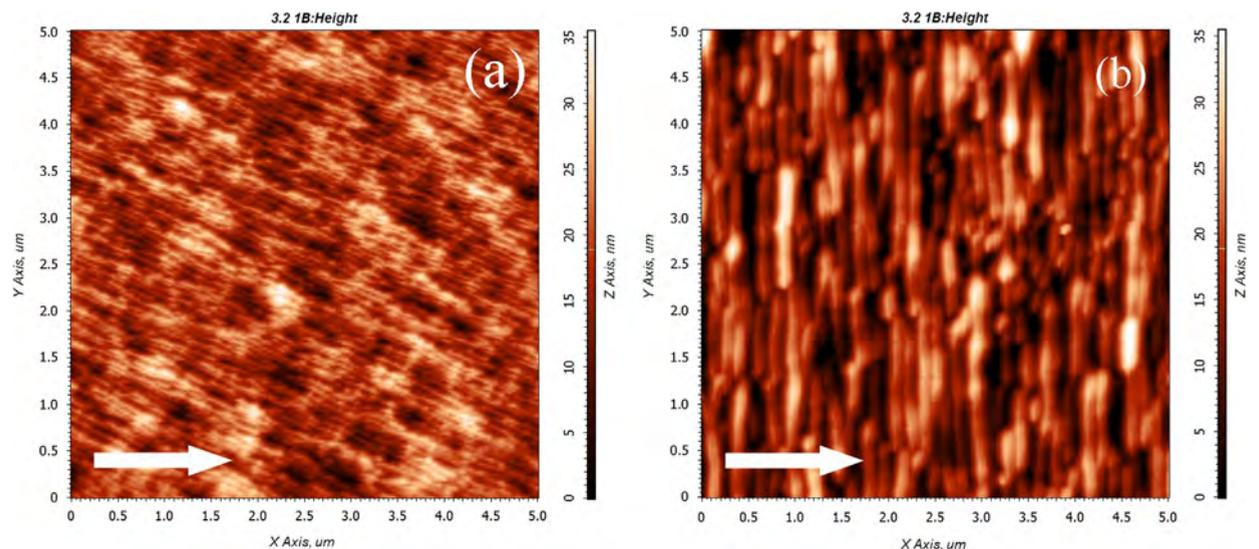
Fig. 1.  $5 \times 5 \mu\text{m}^2$  AFM images of GaAs bombarded with oxygen ions at  $45^\circ$  incidence angle and different ion beam energies: (a) 1 keV, ion fluence is  $6.2 \times 10^{18}$  ions/cm<sup>2</sup>, (b) 2 keV, ion fluence is  $5.4 \times 10^{18}$  ions/cm<sup>2</sup>. The white arrow indicates the direction of the incident ion beam.
