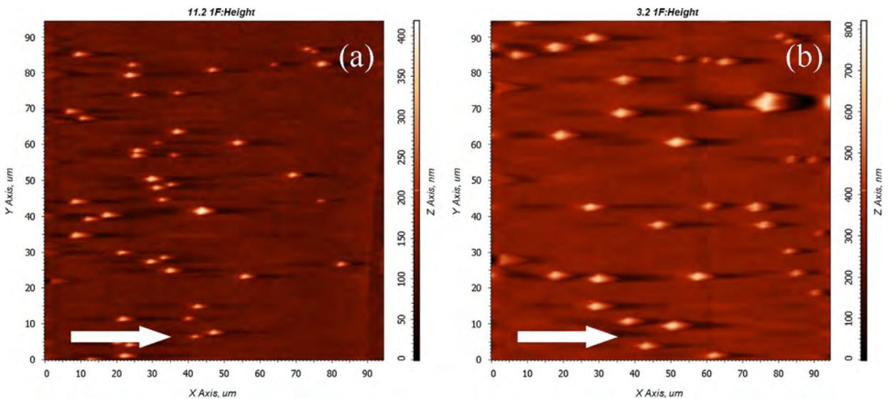
**Fig. 9.** AFM micrographics of InSb bombarded with oxygen ions. The angle of incidence is  $45^\circ$ , the ion beam energy is 1 keV. The ion fluence is:  $3.1 \times 10^{18}$  ions/cm<sup>2</sup> (a) and  $6.2 \times 10^{18}$  ions/cm<sup>2</sup> (b). Image size is  $94.6 \times 94.6 \mu\text{m}^2$ .
