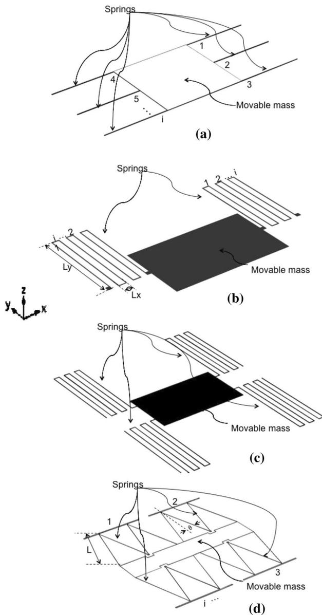
**Fig. 4** Possible configurations for capacitive mobile structure
