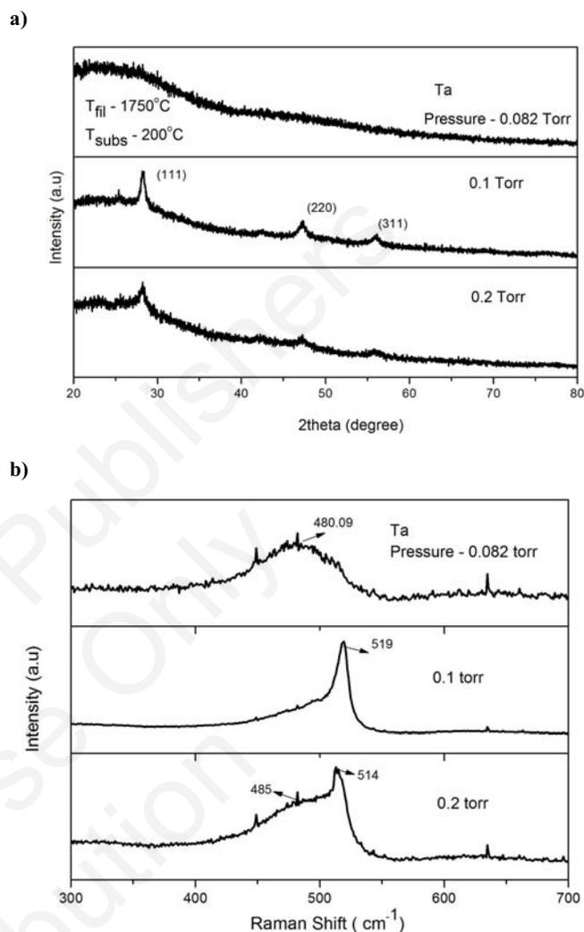
**Fig. (1).** (a) and (b), XRD and Raman spectra, respectively of films deposited with Ta wire, for several process pressures with  $T_{\text{fil}} = 1750^\circ\text{C}$ ,  $T_{\text{subs}} = 200^\circ\text{C}$  and constant  $\text{H}_2/\text{SiH}_4/\text{B}_2\text{H}_6/\text{O}_2 = 5/5/10/0.5$  sccm flow.
