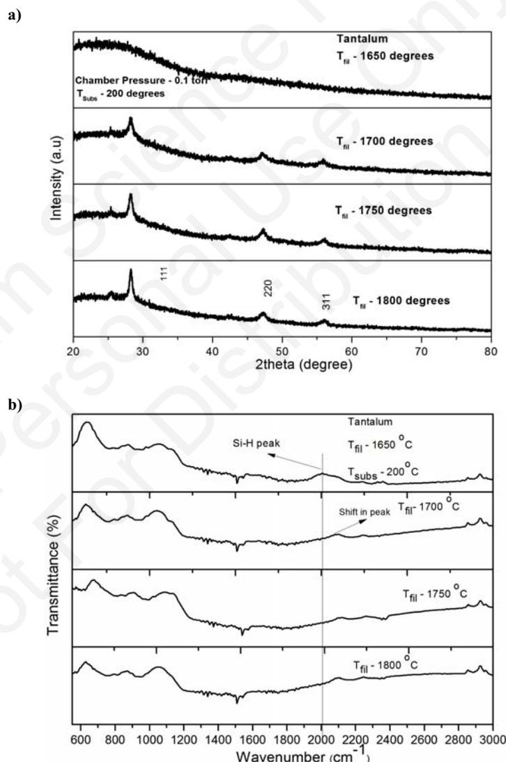
**Fig. (5).** (a) and (b), XRD and FTIR spectra, respectively of samples deposited with Ta wire at different filament temperatures ( $T_{\text{fil}}$ ), with  $\text{H}_2/\text{SiH}_4/\text{B}_2\text{H}_6/\text{O}_2 = 5/5/10/0.5$  sccm flow at 0.1 Torr.
