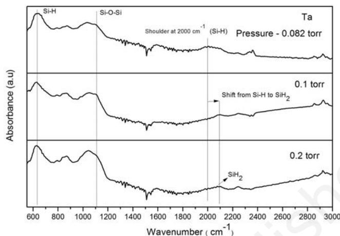
Fig. (2). FTIR spectra of nc-Si/SiO<sub>2</sub> film deposited using HW-CVD at various process pressures.
