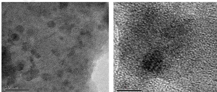
Fig. (4). HRTEM images showing the small nanoparticles of various size distributions at 0.1 and 0.2 Torr.
