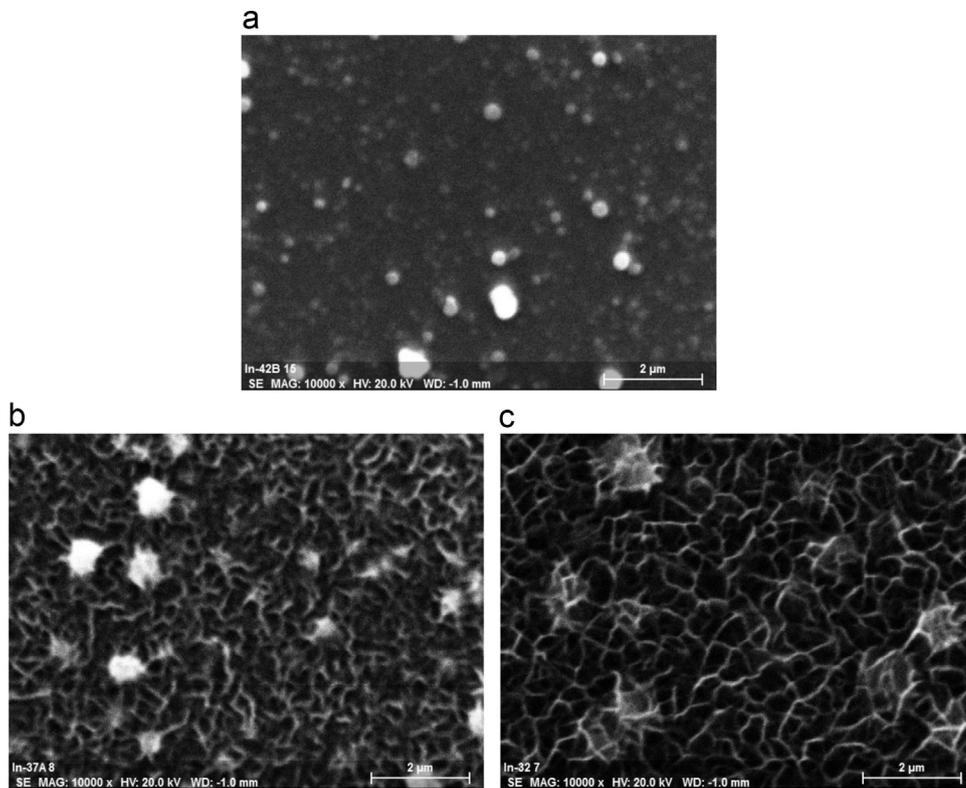
Fig. 3. SEM image of representative CIS samples.
