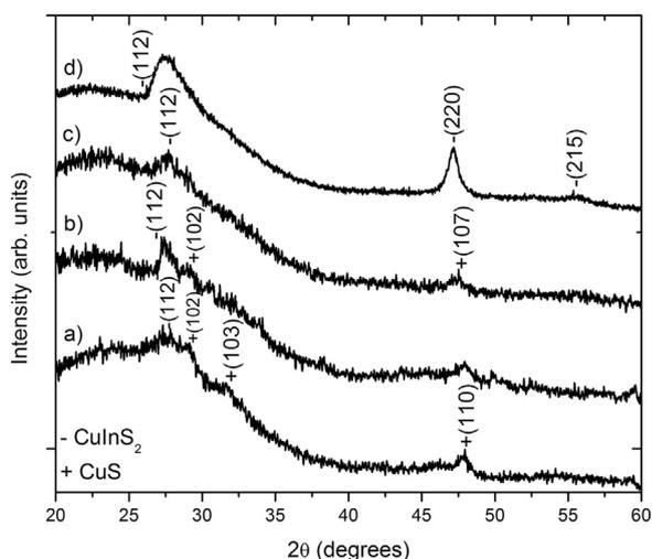
**Fig. 2.** XRD patterns of CIS films. The diffractogram 2(d) confirms the formation of the  $\text{CuInS}_2$  compound.
