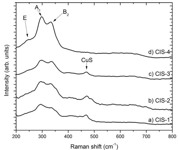
**Fig. 1.** Raman spectra of CIS films grown by CBD. Note the change in the Raman signal as the In nominal concentration increased in bath.
