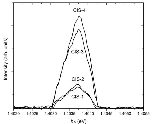
Fig. 4. Photoluminescence spectra at room temperature of CIS films grown by CBD.
