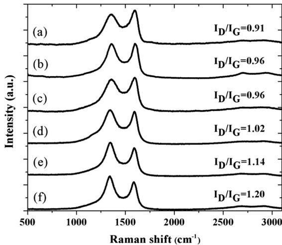
**Fig. 3** Raman spectra of (a) as-deposited GO and annealed samples at (b) 200, (c) 400, (d) 600, (e) 800, and (f) 1000 °C, for 1 h
