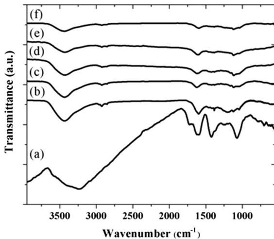
**Fig. 4** FT-IR spectra of (a) the as-deposited GO and (b–f) samples annealed in the temperature range 200–1000 °C
