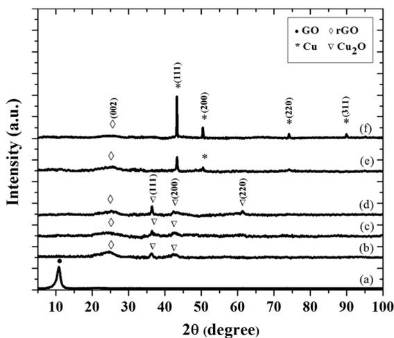
**Fig. 1** XRD patterns of (a) the as-deposited GO and annealed samples at (b) 200, (c) 400, (d) 600, (e) 800, and (f) 1000 °C, for 1 h
