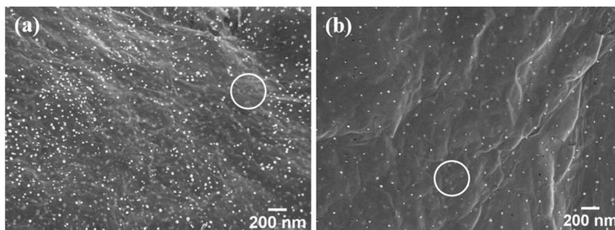
**Fig. 5** FESEM images of samples annealed at (a) 200 and (b) 400 °C, for 1 h. It is seen that the nanocomposite comprises embedded (*circle*) and surfaced  $\text{Cu}_2\text{O}$  nanoparticles in rGO network
