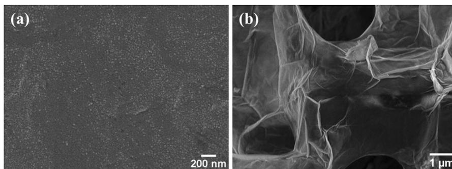
**Fig. 2** FESEM images of (a) the surface Cu foil after being cleaned (b) as-deposited GO on Cu foil after drying at 80 °C
