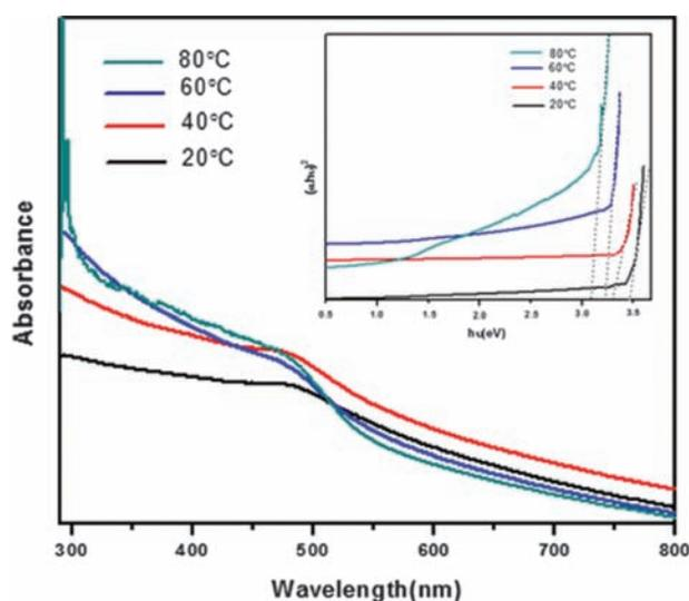
**Figure 7.** UV-visible absorption spectra of the CdS nanoparticles synthesized at different reaction temperature and the inset shows the  $(\alpha h\nu)^2$  versus  $h\nu$  plots with corresponding fitting of the samples.
