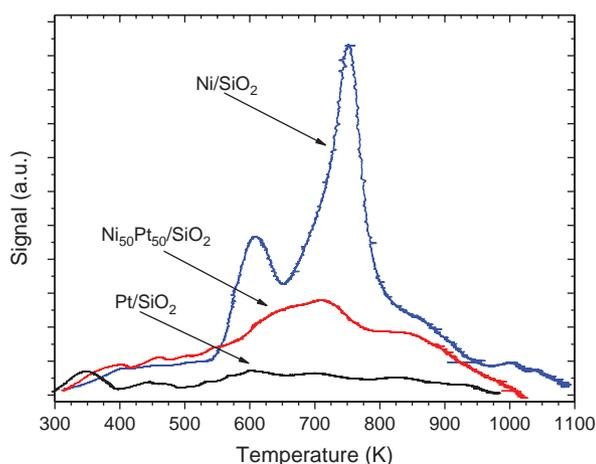
**Figure 6.** TPR profiles of Ni/SiO<sub>2</sub>, Pt/SiO<sub>2</sub> and Ni<sub>50</sub>Pt<sub>50</sub>/SiO<sub>2</sub> catalysts prepared via incipient wetness techniques.
