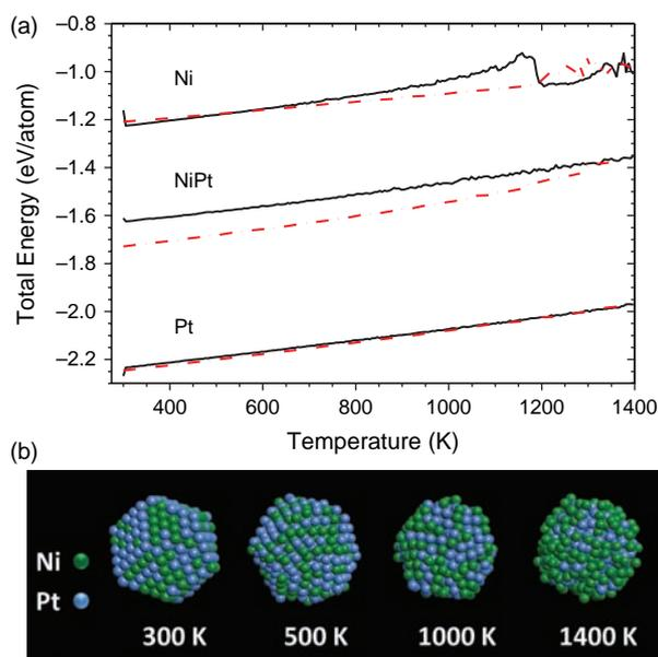
**Figure 8.** (a) Correlation of the total energies with the temperature of the Ni, NiPt and Pt structures. (b) Models of the NiPt particle at different temperatures.
