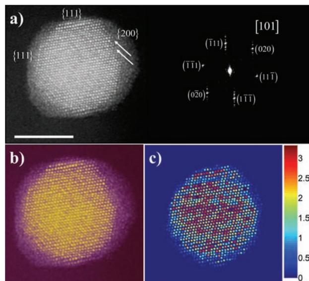
**Figure 5.** (a) HAADF-STEM image with its corresponding FFT, (b) Color look-up HAADF-STEM image, and (c) Map representing integrated intensity of the atoms.
