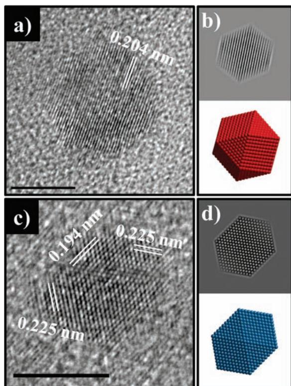
**Figure 2.** HR-TEM images of Ni/SiO<sub>2</sub> and Pt/SiO<sub>2</sub> catalysts. (a) Ni particle with regular shape, (b) simulated image and model of Ni particle, (c) HR-TEM image of Pt particle and (d) simulated image and model of Pt particle.
