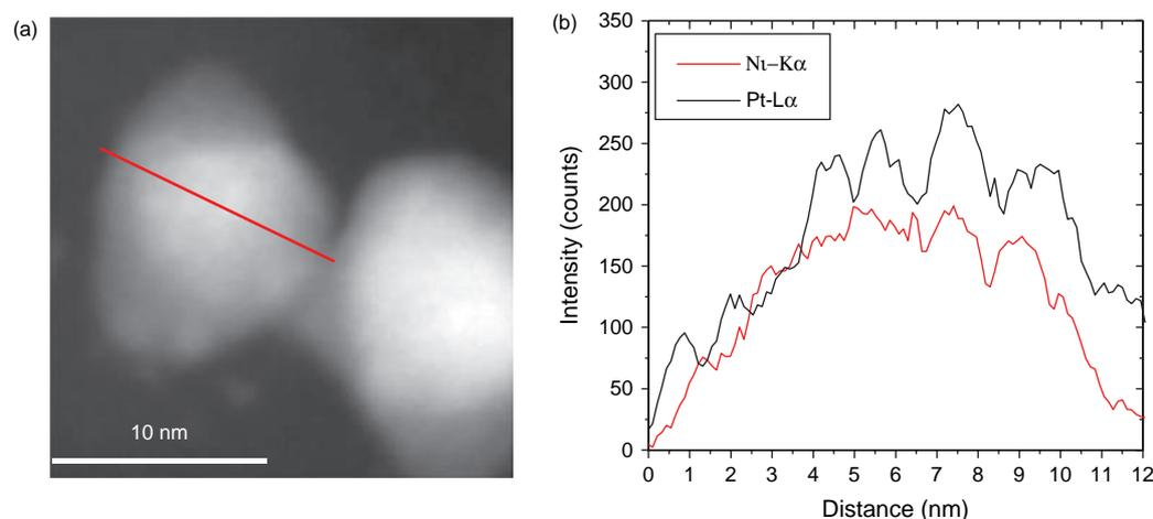
**Figure 4.** STEM-EDS elemental analysis by line-scan across the Ni<sub>50</sub>Pt<sub>50</sub>/SiO<sub>2</sub> catalyst. (a) HAADF-STEM image of the corresponding Ni<sub>50</sub>Pt<sub>50</sub>/SiO<sub>2</sub> catalyst and (b) Elemental Ni and Pt line profiles, the overlapping indicates homogeneous alloy distribution in the catalysts.
