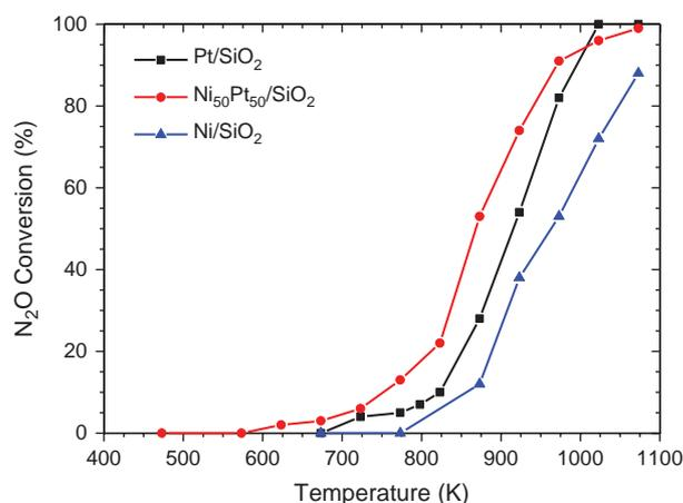
**Figure 7.** Catalytic activity profiles for catalyst of Ni/SiO<sub>2</sub>, Pt/SiO<sub>2</sub> and Ni<sub>50</sub>Pt<sub>50</sub>/SiO<sub>2</sub> during the decomposition of N<sub>2</sub>O gas.
