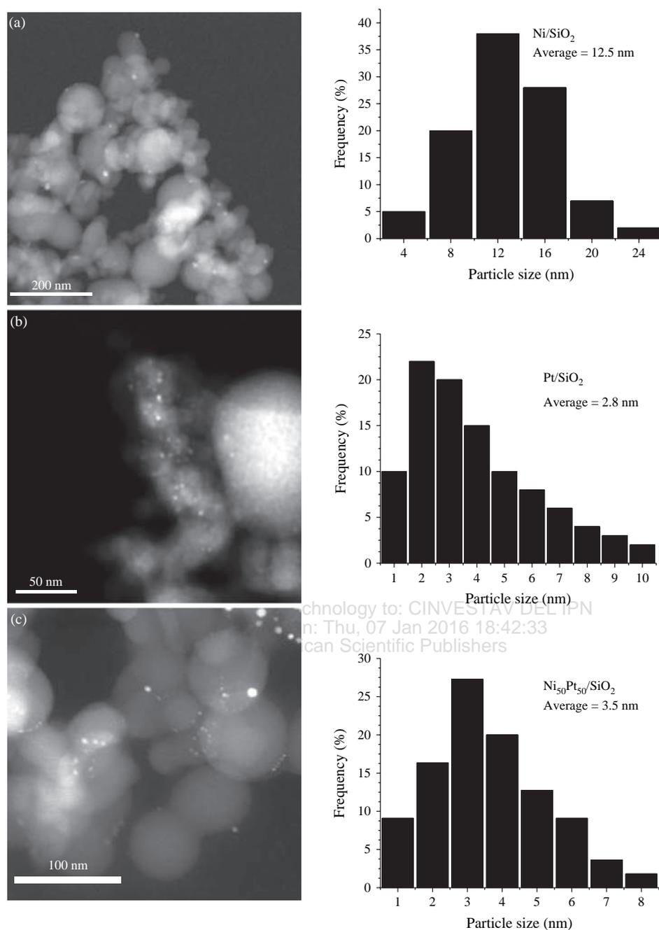
**Figure 1.** STEM images and particle size histograms of: (a) Ni/SiO<sub>2</sub>, (b) Pt/SiO<sub>2</sub> and (c) Ni<sub>50</sub>Pt<sub>50</sub>/SiO<sub>2</sub>.
