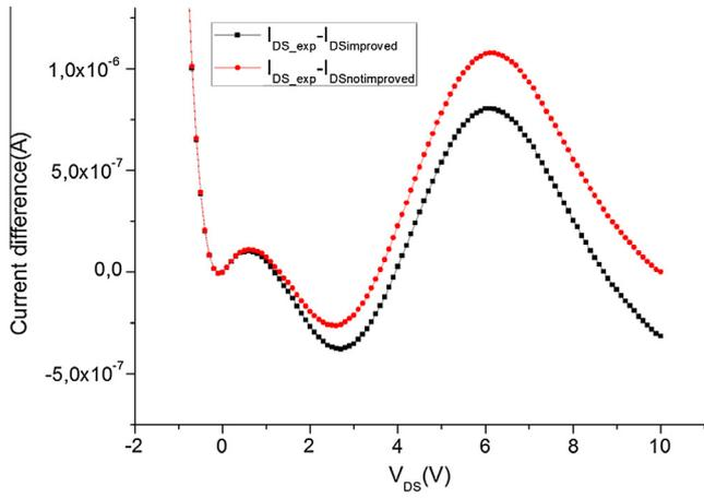
Fig. 2. The difference between the measured current ( $I_{DS\_exp}$ ), the model with improvement ( $I_{DSImproved}$ ) and the model without improvement ( $I_{DSNotImproved}$ ) for  $V_{GS} = 8V$ .
