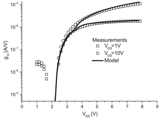
Fig. 6. Transconductance characteristics. Model (lines) and measurements (symbols).
