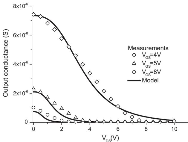
Fig. 4. Output conductance characteristics. Model (lines) and measurements (symbols).
