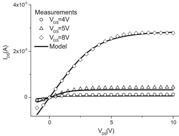
Fig. 3. Output characteristics. Model (lines) and measurements (symbols).
