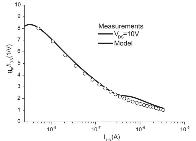
Fig. 7. Calculated and measured  $g_m/I_{DS}$  versus  $I_{DS}$ . Model (lines) and measurements (symbols).
