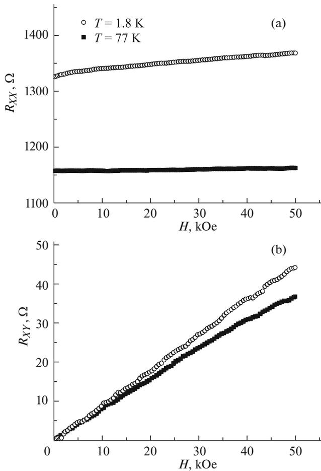
**Fig. 2.** Dependences of the (a) longitudinal and (b) Hall resistances on the external magnetic field of the GaAs : Be/Ga<sub>0.84</sub>In<sub>0.16</sub>As/GaAs/ $\delta$ -Mn/GaAs heterostructure with a  $\delta$ -layer 1.2 ML thick at  $T = 1.8$  K (open circles) and  $T = 77$  K (closed squares).
