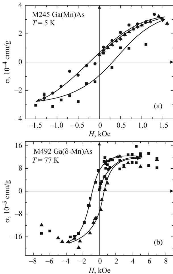
**Fig. 4.** Magnetic-field dependences of the specific magnetization for (a) the GaAs/Ga<sub>0.84</sub>In<sub>0.16</sub>As/Ga(Mn)As heterostructure and for (b) the GaAs : Be/Ga<sub>0.84</sub>In<sub>0.16</sub>As/GaAs/( $\delta$ -Mn/GaAs heterostructure with a  $\delta$ -layer 1.2 ML thick.
