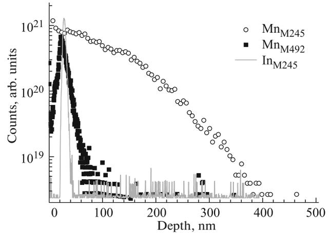
**Fig. 1.** Experimental manganese distribution profiles in sample *A* (open circles) and sample *B* (closed squares) in the epitaxial growth direction, measured by secondary ion mass spectrometry (SIMS) using a Cameca ims-6f ion microprobe. The gray solid curve is the indium distribution profile, i.e., the GaAs/InGaAs/GaAs quantum well profile. The horizontal axis zero corresponds to the air/sample surface interface.
