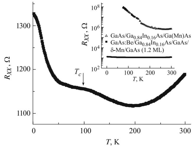
**Fig. 3.** Temperature dependence of the longitudinal resistance in the GaAs/Ga<sub>0.84</sub>In<sub>0.16</sub>As/GaAs/ $\delta$ -Mn/GaAs heterostructure doped with a manganese  $\delta$ -layer 1.2 ML thick. The inset shows the dependences  $R_{XX}(T)$  for heterostructures with a Ga(Mn)As layer (open triangles) and a manganese  $\delta$ -layer (closed squares).
