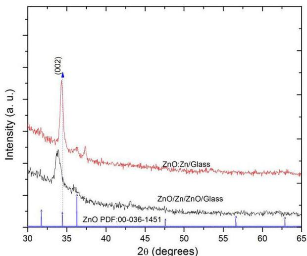
FIGURE 3. XRD patterns of the as-deposited ZnO/Zn/ZnO/Glass structure and the ZnO:Zn(n<sup>+</sup>) films.
