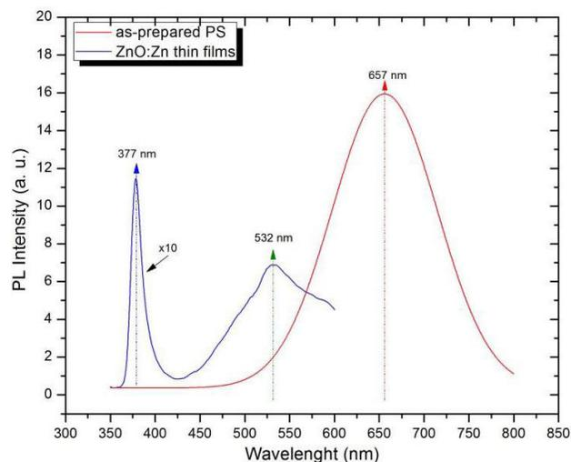
FIGURE 2. Room temperature PL spectrum of; a) an as-prepared PS film and b) a ZnO:Zn(n<sup>+</sup>) thin film.
