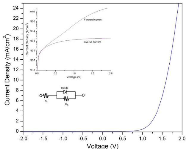
FIGURE 4. I-V characteristics of the ZnO:Zn(n<sup>+</sup>)/PS/Si(p) heterojunction. The insets are a semi-log I-V characteristic and an equivalent electrical circuit.
