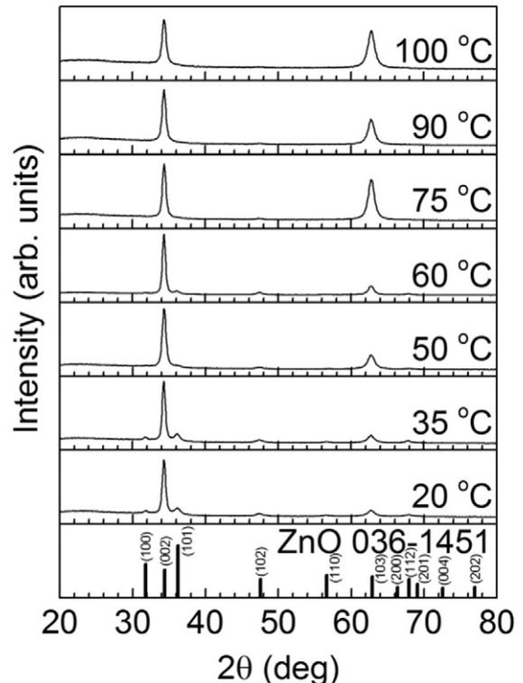
Fig. 1. XRD spectra of the AZO films deposited at different substrate temperatures.
