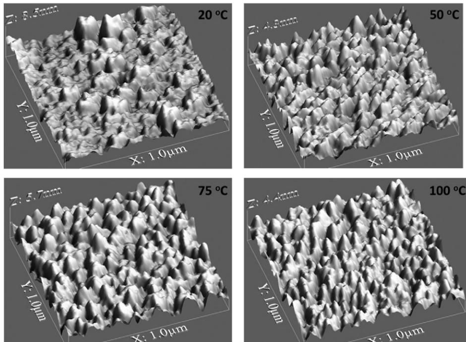
**Fig. 2.** AFM 3D images for the films deposited at 20, 50, 75 and 100 °C.
