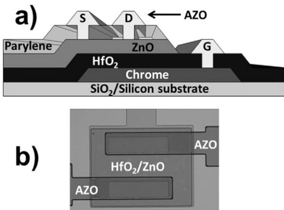
Fig. 6. a) Schematics of the fabricated TFTs. b) Optical microscope image of the completed device ( $W = 80 \mu\text{m}$  and  $L = 40 \mu\text{m}$ ).
