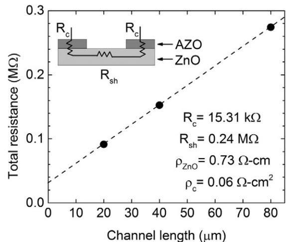
Fig. 8. Transfer length method used for estimating  $R_c$  and  $\rho_c$ . The inset shows the composition of the total resistance.
