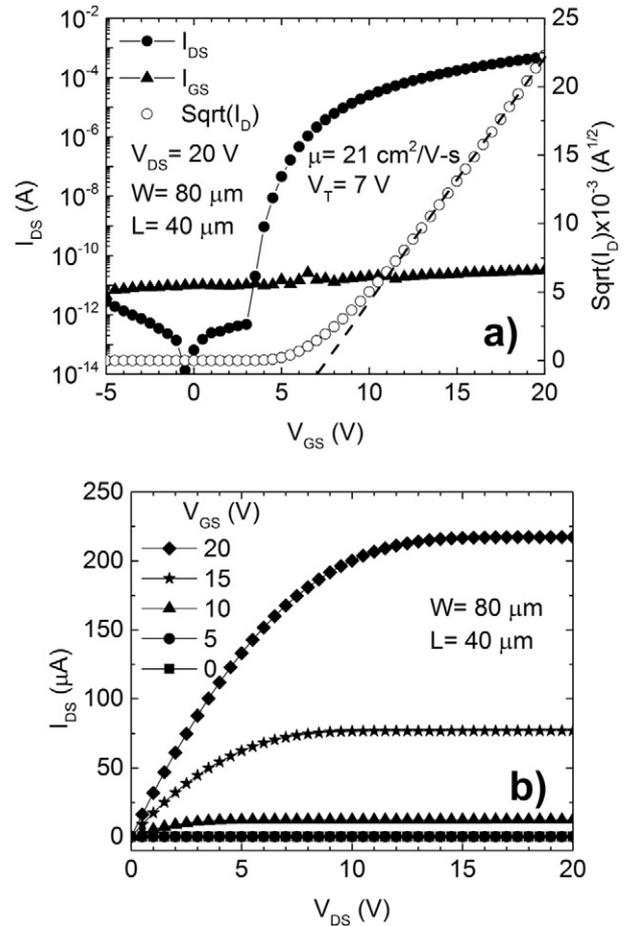
Fig. 7. a)  $I_{DS}$ - $V_{GS}$  and b)  $I_{DS}$ - $V_{DS}$  plots of the fabricated devices ( $W = 80 \mu\text{m}$  and  $L = 40 \mu\text{m}$ ).
