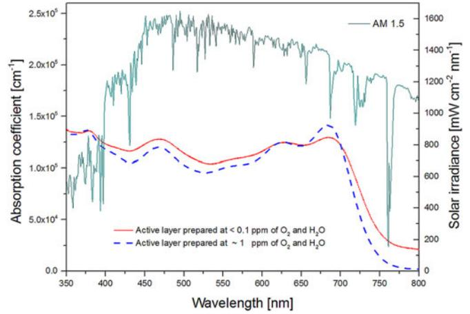
Fig. 5. Absorption coefficient of PTB7:PC<sub>70</sub>BM blend layers manufactured under a nitrogen environment with H<sub>2</sub>O and O<sub>2</sub> < 0.1 ppm (red solid line) and H<sub>2</sub>O and O<sub>2</sub> ~ 1 ppm conditions (blue dashed line). The solar irradiance under AM 1.5 is shown in the same graph.
