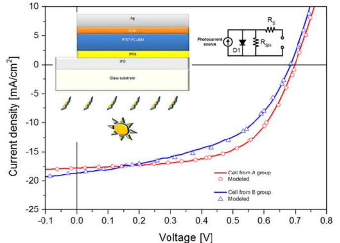
Fig. 1. Current-voltage ( $J$ - $V$ ) characteristics of PTB7:PC<sub>70</sub>BM inverted OSCs from A and B groups under  $100 \text{ mW}/\text{cm}^2$  equivalent illumination intensity corresponding to AM 1.5G sun light standard. (Inset) Device structure and the equivalent circuit used. Measured characteristics (solid lines) and modeled characteristics (open symbols).
