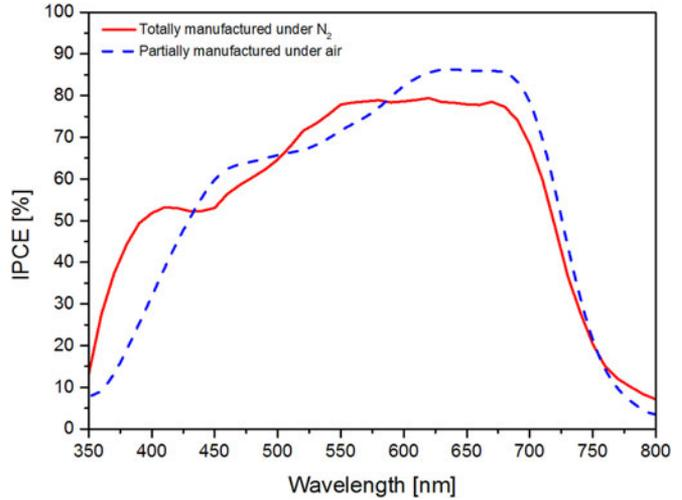
Fig. 6. IPCE spectrum of inverted OSCs from A group totally manufactured under N<sub>2</sub> and B group partially manufactured under air conditions. The IPCE was just measured after sample fabrication.
