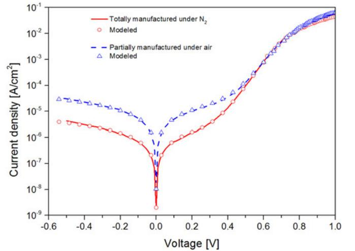
Fig. 2. Semi-log  $J$ – $V$  curve under darkness for both groups of cells manufactured. Measured characteristics (solid lines) and modeled characteristics (open symbols).
