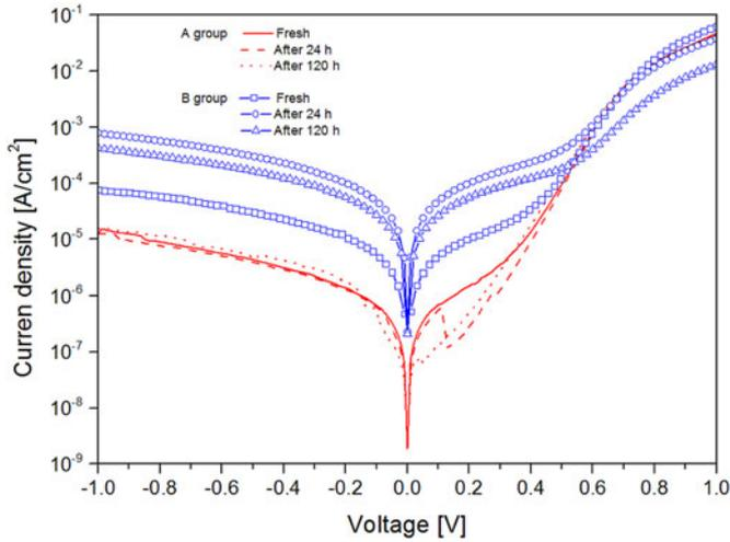
Fig. 4. Degradation with time of semi-log  $J$ - $V$  curves under dark of inverted PTB7:PC<sub>70</sub>BM solar cells for the A group (devices fabricated under an N<sub>2</sub> environment) and for the B group (devices partially fabricated under air). Samples were kept under a nitrogen environment between measurements.
