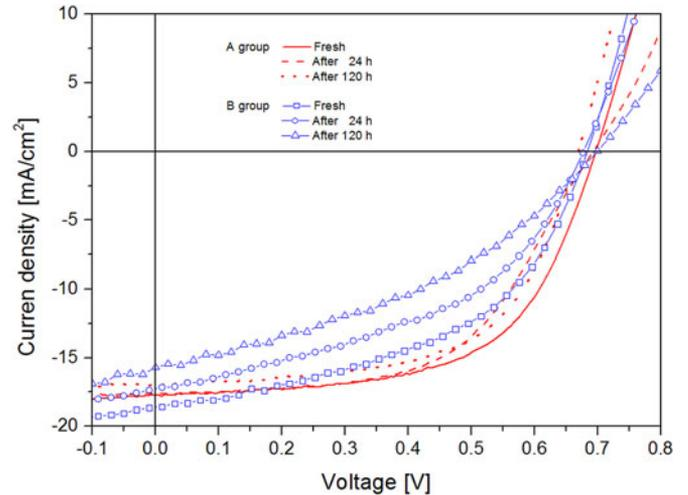
Fig. 3. Illuminated  $J$ - $V$  curves of inverted PTB7:PC<sub>70</sub>BM solar cells for the A group (devices fabricated under a N<sub>2</sub> environment) and for the B group (devices partially fabricated under air) for different degradation times under a nitrogen environment during 120 h. All the devices were measured under AM 1.5G spectrum condition (100 mW/cm<sup>2</sup>).
