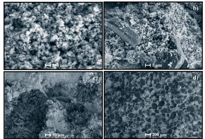
Fig. 3. SEM images of  $\text{SnO}_2$  and  $\text{Al}_2\text{O}_3$  mixed pellets surface at magnification of (a) 200nm, (b)  $1\mu\text{m}$ , (c)  $10\mu\text{m}$ , and (d)  $200\mu\text{m}$ .
