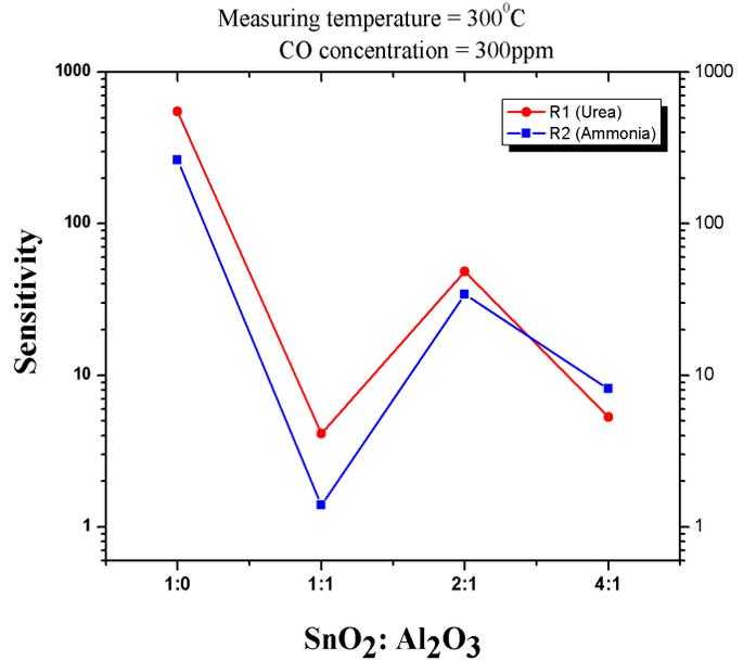
Fig. 1. Comparison of sensitivities of SnO<sub>2</sub>: Al<sub>2</sub>O<sub>3</sub> pellets for different mixing ratios.
