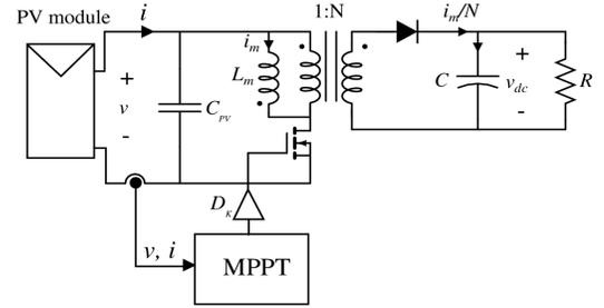
Fig. 2. The DC-DC stage.
