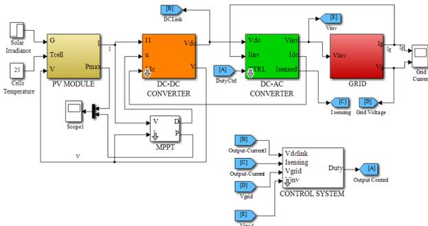
Fig. 8. Simulink model of the proposed micro-inverter
