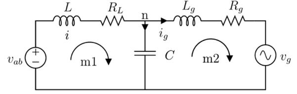
Fig. 5. Equivalent circuit for the DC-AC stage.
