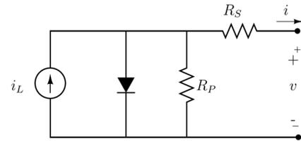
Fig. 3. PV module equivalent circuit [24].
