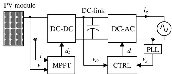
Fig. 1. Double stage micro-inverter.
