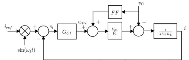
Fig. 6. Block diagram for the current control loop [29].
