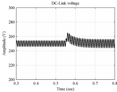
Fig. 10. Voltage regulation at the DC-link.
