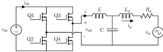
Fig. 4. The DC-AC stage.
