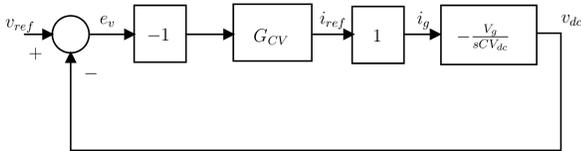
Fig. 7. Block diagram for the voltage control-loop [29].
