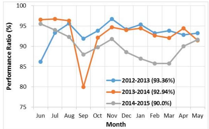
Fig. 5. Measured PR of the PV system during 36 months. The corresponding average PR for the period is indicated in the parenthesis.
