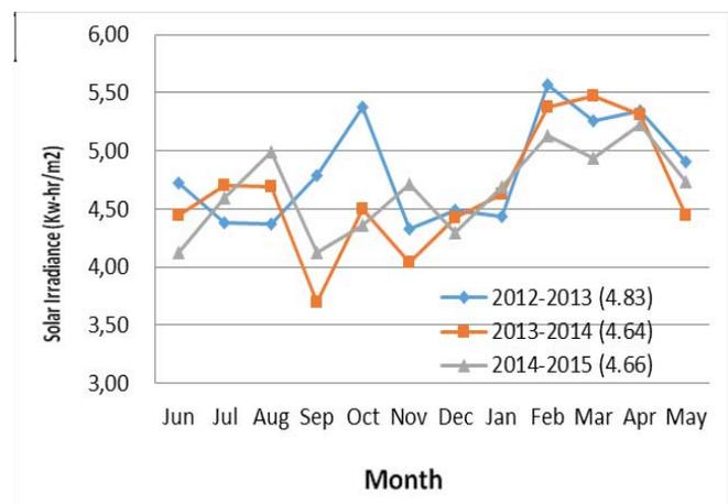
Fig. 2. Monthly average Solar irradiance measured at POA by using c-Si solar cell sensor, which is monitored by Fronius inverter system. The irradiance units were kWh/m<sup>2</sup>/day. The number in the parenthesis indicates the average irradiance during the measured period in peak-hours (or kWh/m<sup>2</sup>).
