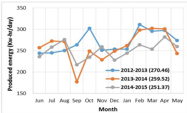
Fig. 4. Monthly-based average produced energy from the PV system. The number in the parenthesis indicates the produced daily average energy during the indicated period in kWh/day.
