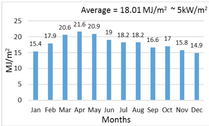
Fig. 6. Monthly averaged solar radiation from January to December during fourteen (1999-2012) consecutive years. The irradiation was measured by using horizontal pyranometer [3].
