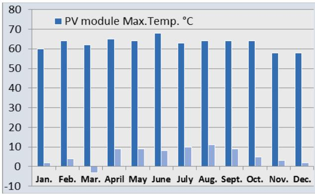
Fig. 3. Maximum and minimum PV module temperatures (in °C) during 2013.
