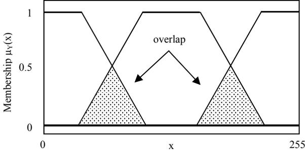
Fig.4. Overlap in fuzzy sets, inaccurate transition of the hue.
