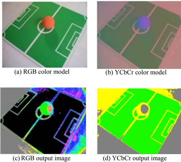
Fig. 10. Segmentation process in the RGB and YCbCr color spaces, (a) Original image in RGB color space, (b) Original image transformation into YCbCr color space, (c) Segmentation of green color in RGB, (d) Segmentation of green color in YCbCr.
